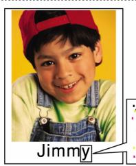
Toner is splattered in the image, depending on the type of paper, used.
